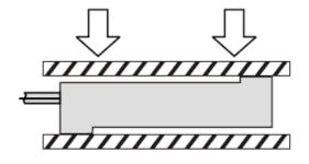
ARROW SHOWS LOAD DIRECTION FOR +VE OUTPUT
